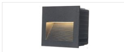
IP65 Square recessed wall light GR-BD-L-05 / 9W-12W 15W 18W options L160*W160*H65mm, cutout:155*155mm
