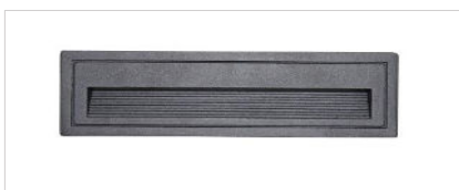
Rectangle wall light IP65 GR-BD-L-02 / 5W 100-240VAC 50/60Hz L210*W60*H55mm, Cutout:205*55mm
