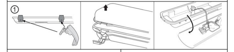
Screw two pieces metal bracket (packed in the accessory bag) to ceiling; install the housing to the metal bracket.
